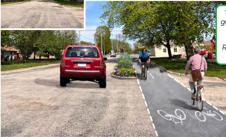
Proposed on-street bike lane with a bioswale buffer along SW B Avenue.
