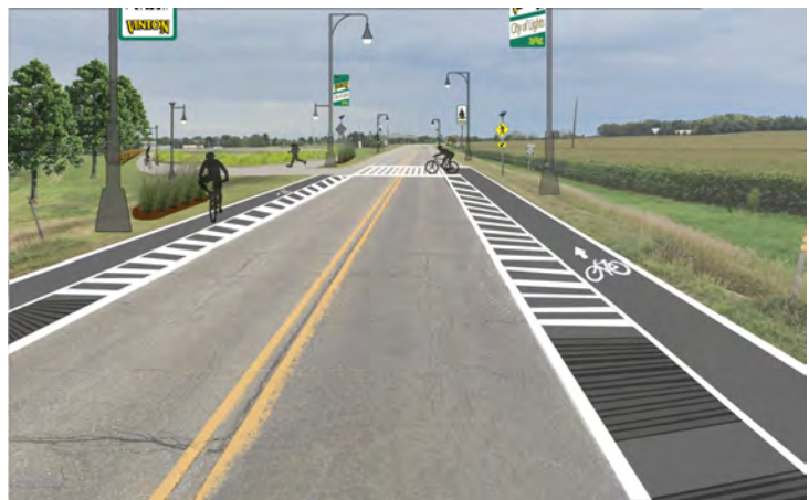
Image edit showing trail option 1—a paved road-shoulder bike lane—for the Highway 218 corridor.
