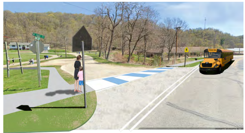
Image edit showing the proposed sidewalk, crosswalk, and pedestrian signage at Turner Park.
