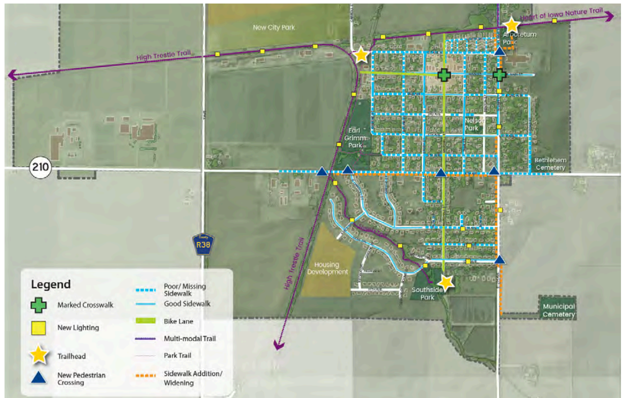
Connectivity plan showing locations for bike lanes, new and wider sidewalks, and new pedestrian crossings.
