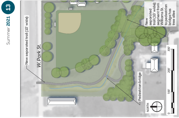
Partial concept plan 13h: The plan above shows an alternate route for the 10' wide separated trail on the northwest portion of the park
