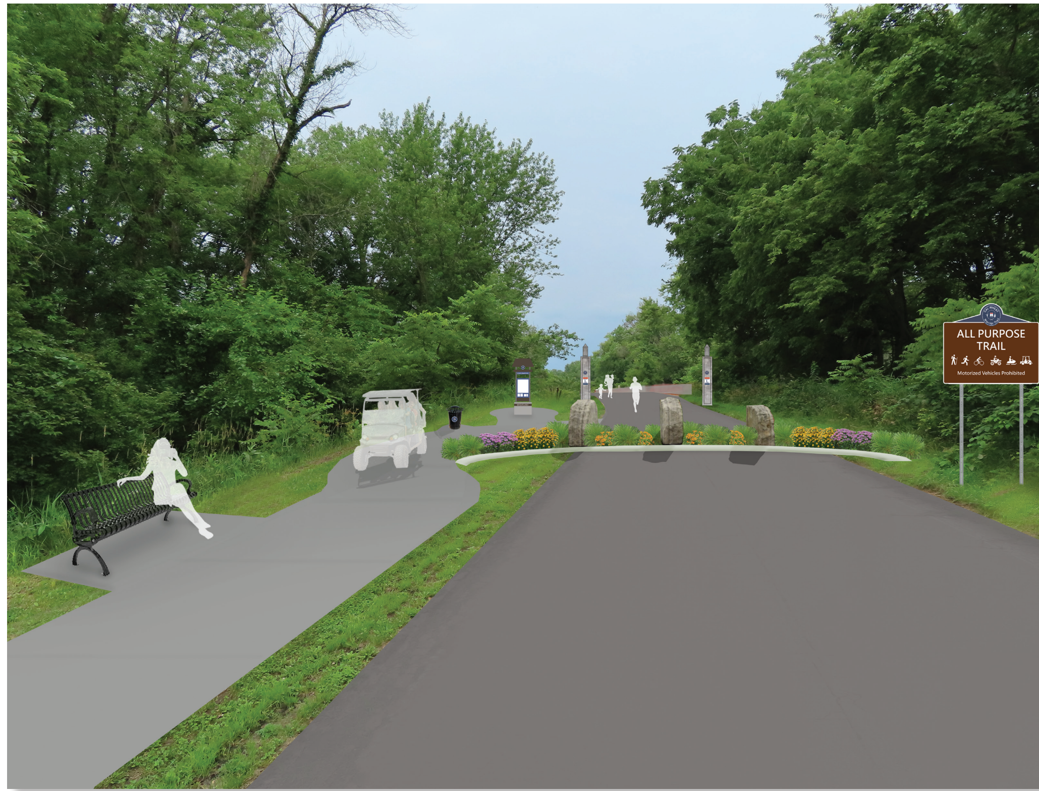
Photo edit 3d: Proposed vehicular barrier access treatment for each end of Wapsi bridge
