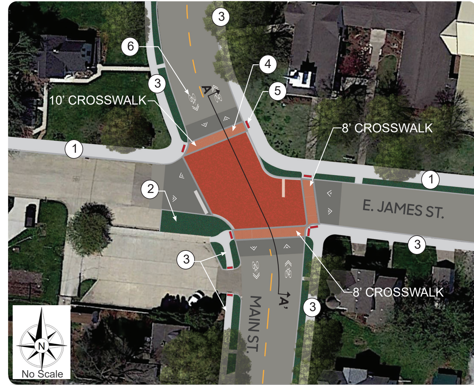
Proposed Concept Plan A utilizing a raised intersection (recommended). See Typical Section A-A' and refer to proposed concept illustration.
