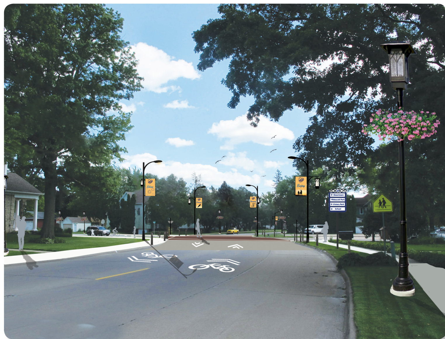
Image edit showing vision for Proposed Concept A (raised intersection). Also illustrated is the proposed continuation of decorative pedestrian lighting with banners and hanging baskets, vehicular lighting, way-finding signage, bollard lighting, and Sharrow markings along Main St.
