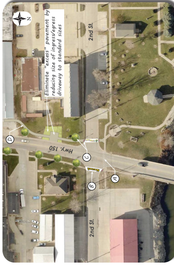
Proposed concept illustrates the following enhancements: 6-foot-wide ADA-compliant sidewalk, pre-fabricated pedestrian bridge, branched way-finding signage, decorative pedestrian lighting with banners, right-of-way planted with native prairie grasses and forbs, with water-tolerant areas planted with appropriate native wet prairie wetland vegetation such as prairie cord grass.
