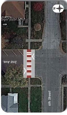
Plan view of proposed raised crosswalk with brick
