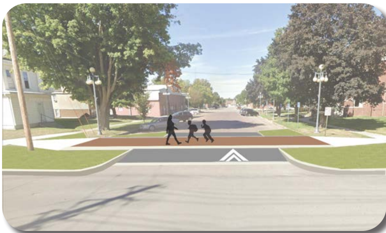
Proposed concept showing brick crosswalk and concrete ramps
