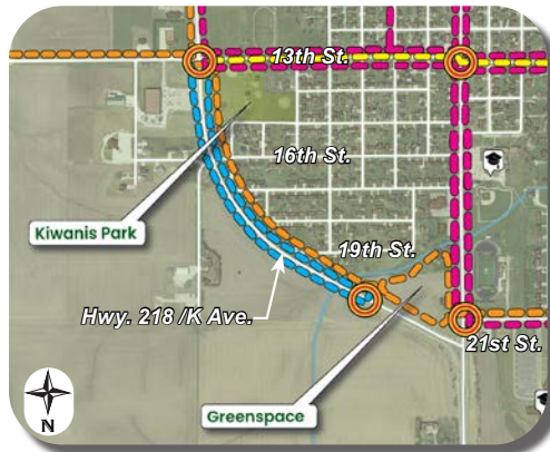
Excerpt from the proposed pedestrian circulation map shown on board 9a. This illustrates the location for the paved shoulder bike lane that is proposed to be an interim segment until a separated trail can be installed in this area as shown on the above excerpt.
