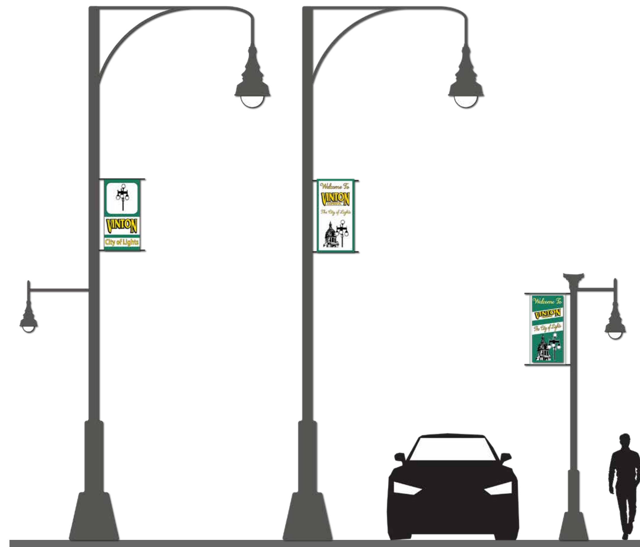
Decorative lighting with banners proposed for major corridors, including Hwy. 218, C Ave., and 3rd & 4th St. from Hwy 218 to downtown. The lights will include pedestrian & vehicular combination, vehicular only, and pedestrian only, as shown above - the type used will depend on the location.
