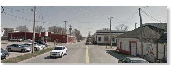
Traveling south, the parking along the west side of Eyberg Avenue becomes a right-hand turn lane. On the east side of the road some curb extension is proposed to allow for widening the fitness center parking lot, adding a north-south sidewalk, and providing a vegetated buffer. A significant shoulder width will be provided along Eyberg Avenue on the east side, especially at the corner, to increase ease of turns for larger vehicles from HWY 92 onto Eyberg Avenue.
