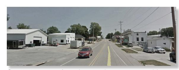
Coming into town from the west, bump-outs would be implemented along both shoulders. This will allow for managing stormwater issues within this area, and providing sidewalk access on the north side of HWY92 where there currently is none. As you approach the "four-corners" the downtown identity elements such as pedestrian street lights would begin to establish the character for this district.
