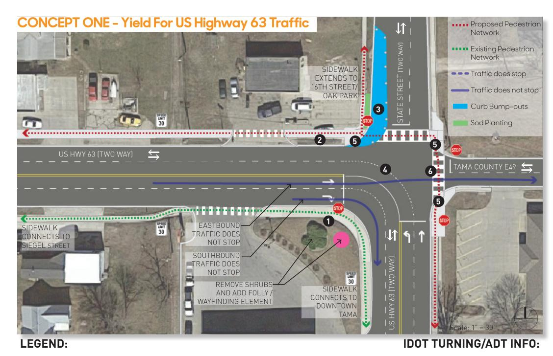
1 Flashing Yield Sign - Slightly slows down US Highway 63 traffic, making drivers aware of potential pedestrians while not requiring a stop to continue onto Highway 63.
