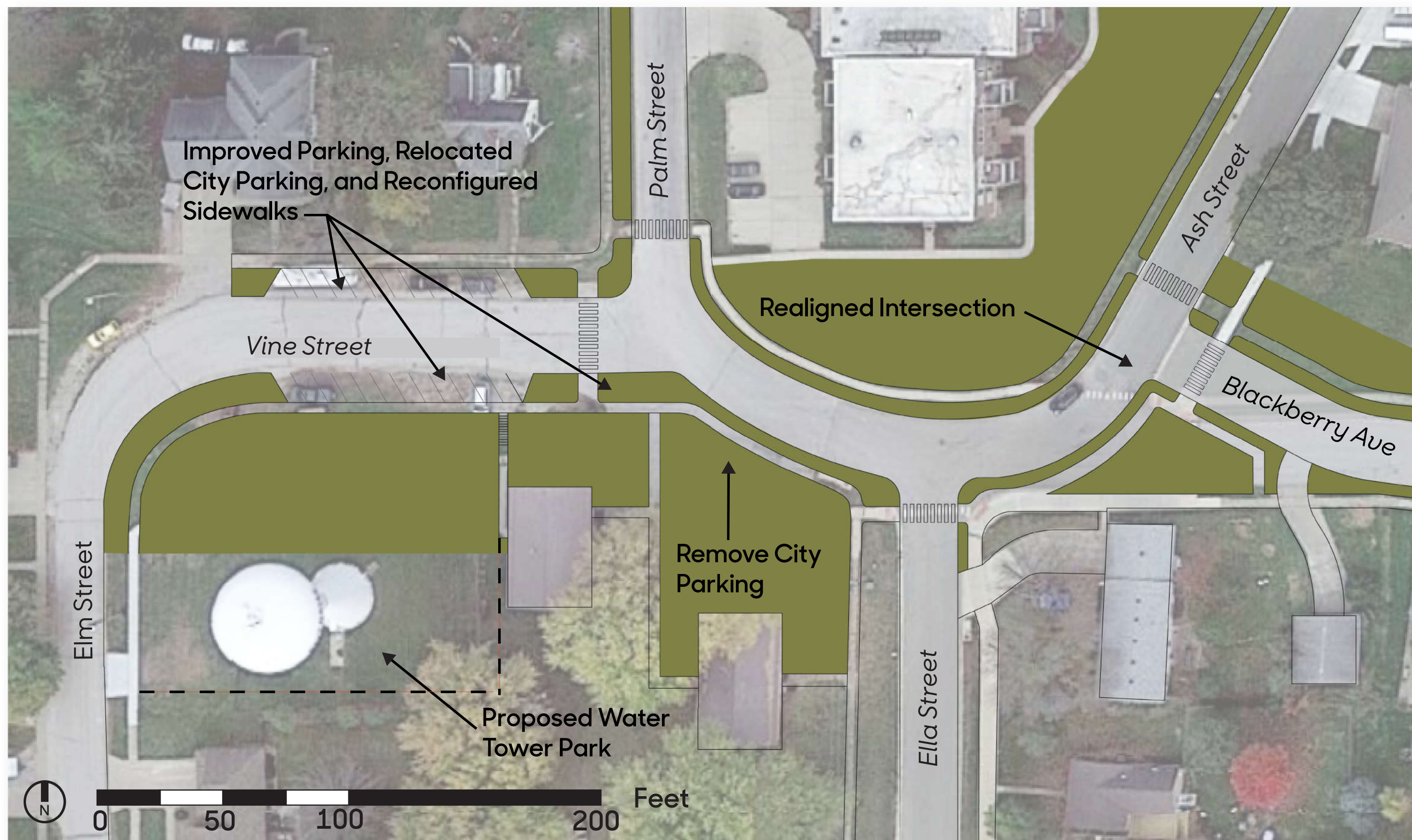
Proposed intersection reconfiguration and infrastructure updates
