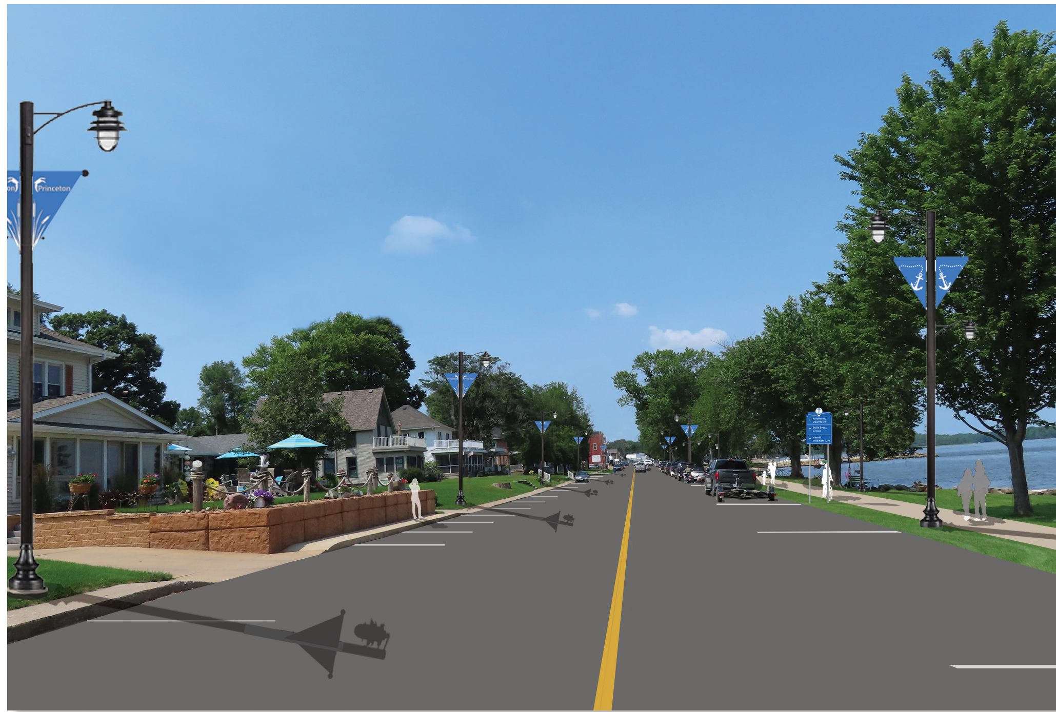
Concept 13c: Enhancements illustrated include decorative lighting (Candela style), underground utilities, paved parking for boaters, separated riverfront recreational trail, new pavement and the associated pavement markings, way-finding signage, and a grass boulevard between the parking and trail. Based on preliminary information publicly available, it appears that the existing road right-of-way is wide enough in this area to accommodate the improvements shown. Concept 13e is the same as this concept except for the lighting style shown; Concept 13d below is the same concept as this one except that the trailer parking utilizes a "green" parking solution like shown in figures 13a and 13b.
