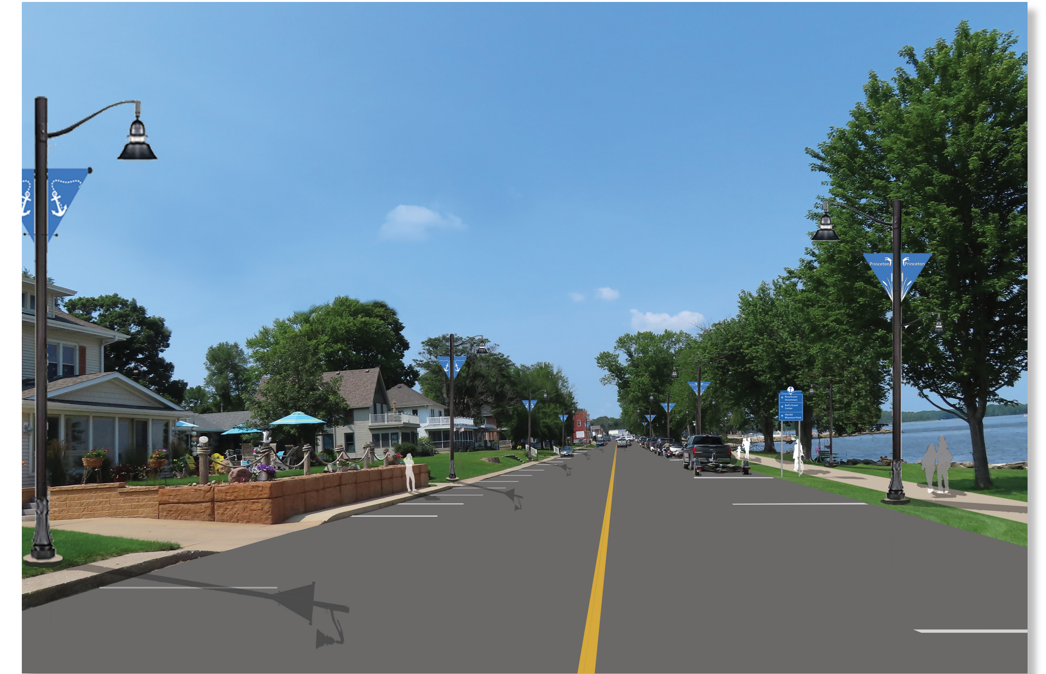
Concept 13e: Enhancements illustrated include decorative lighting (Domus style), underground utilities, paved parking for boaters, separated riverfront recreational trail, new pavement and the associated pavement markings, way-finding signage, and a grass boulevard between the parking and trail. Based on preliminary information publicly available, it appears that the existing road right-of-way is wide enough in this area to accommodate the improvements shown. Concept 13c is the same as this concept except for the lighting style shown; Concept 13f below is the same concept as this one except that the trailer parking utilizes a "green" parking solution like shown in figures 13a and 13b.
