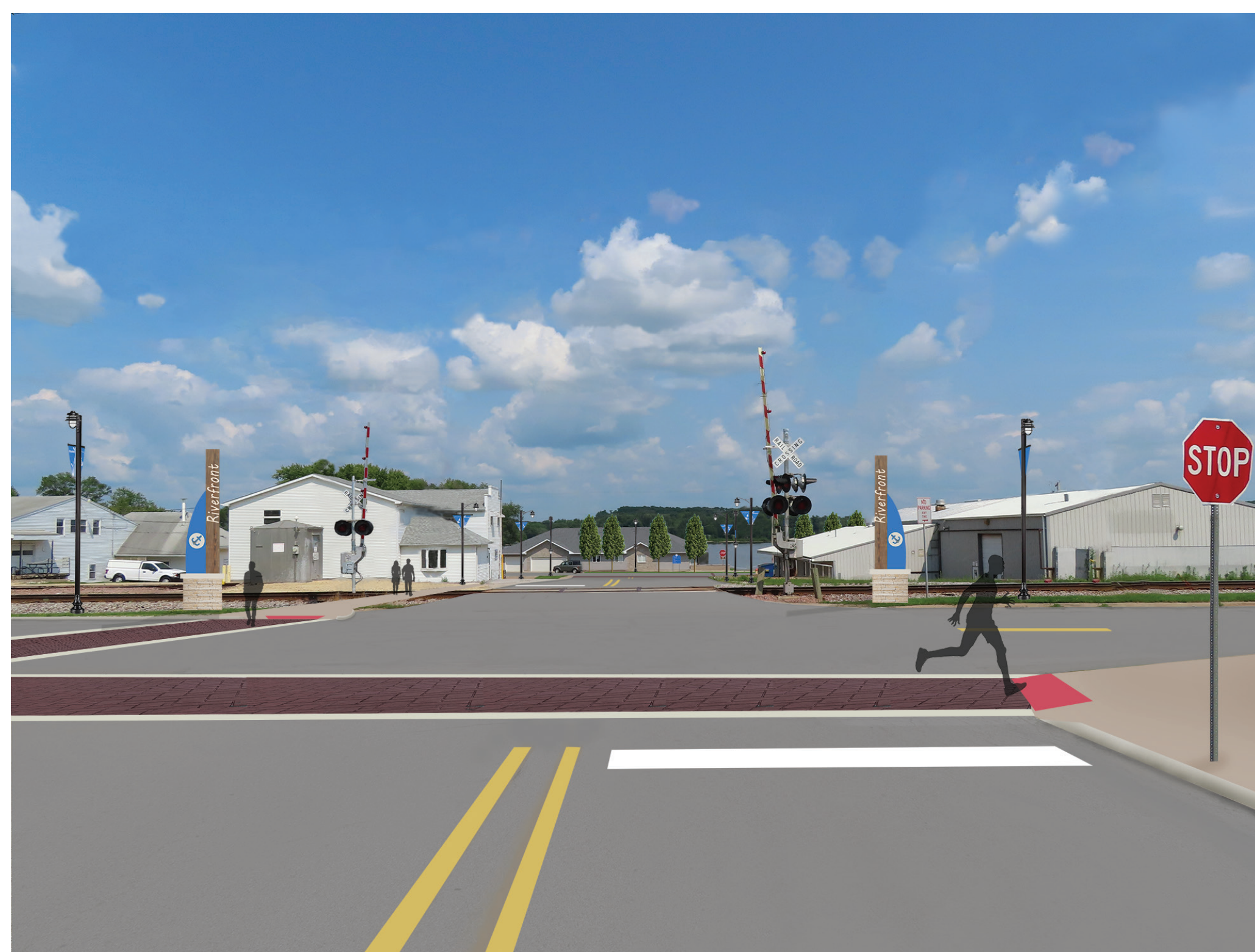
Concept 11a: Riverfront gateway enhancements include decorative pavement for crosswalks, gateway monument (option A3), decorative lighting (candella style), ADA compliant sidewalks
