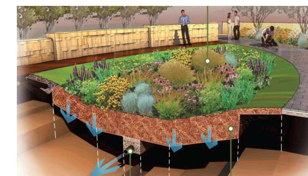
Diagrammatic section-perspective of a bioswale
