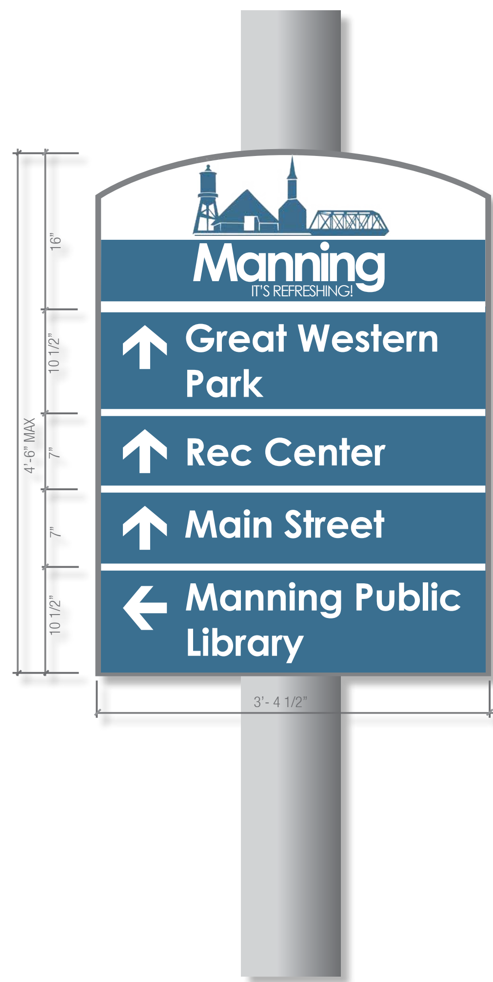
Proposed MUTCD Compliant 3M Reflective Signage
