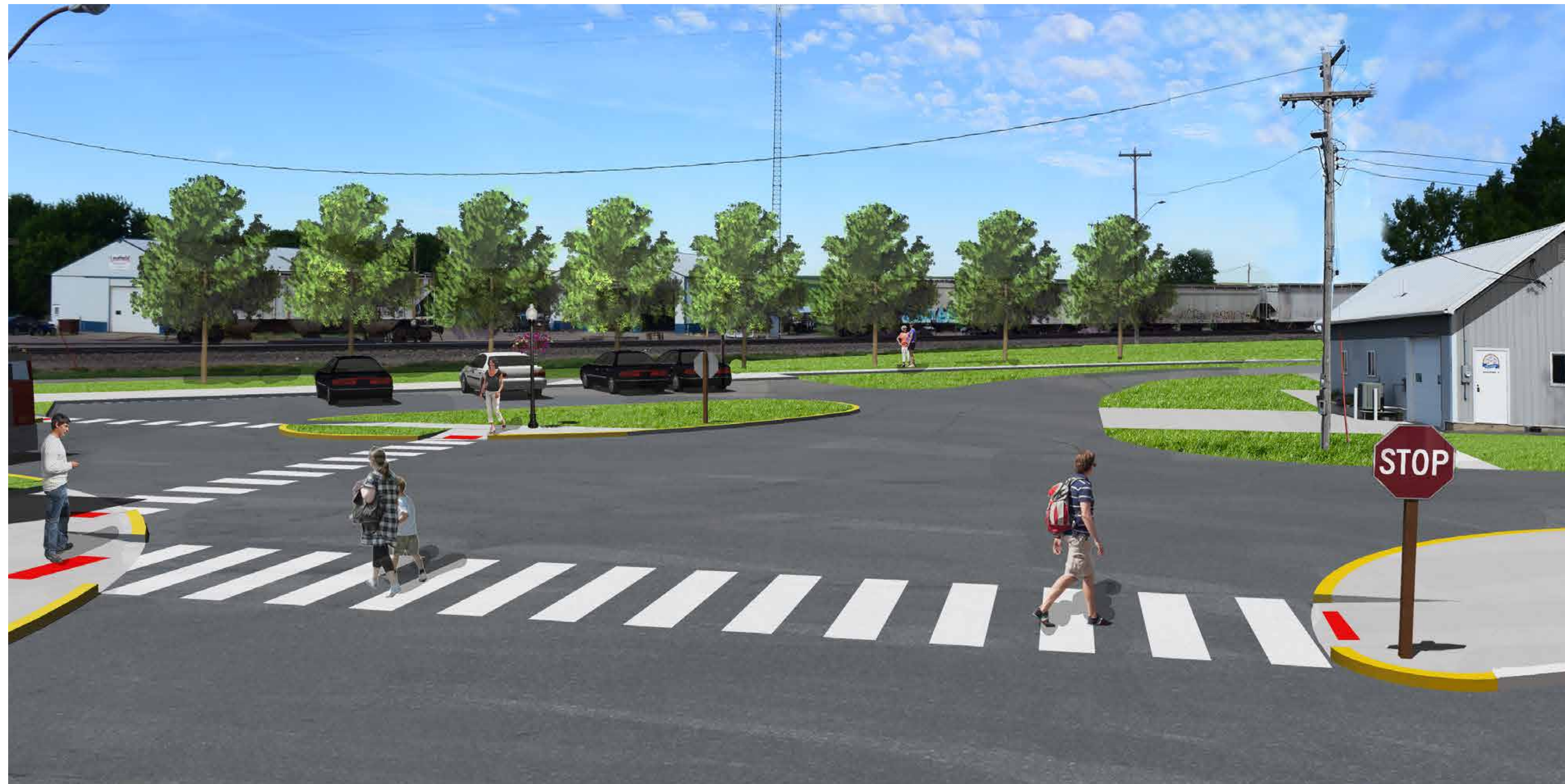
Proposed intersection improvements include bump-outs on Main Street, creating parking space in the existing gravel area along Hastings Street, and improving the turning radius on Hastings Street. Highly visible crosswalks and detectable warning panels on Clinton and Main Streets create a pedestrian friendly environment. A proposed 10' recreational trail next to tree plantings along Hastings Street connect to a proposed sidewalk and at-grade pedestrian railroad crossings leading to the Roy G. Hoogveen Field and Park.
