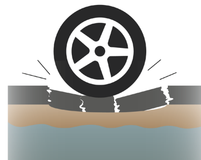
Traffic breaks bubble and wears surface
