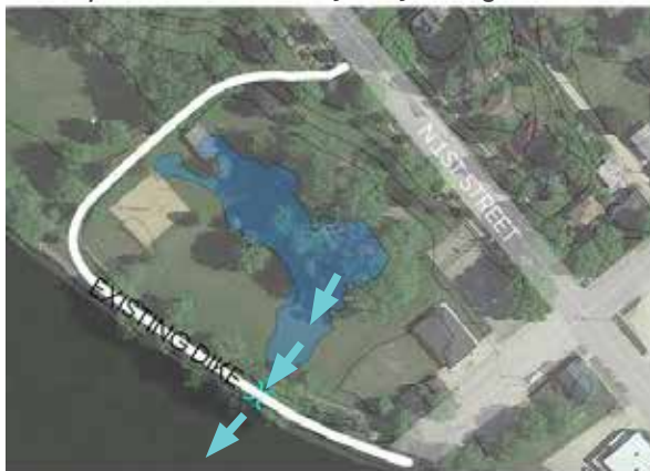
Installing a culvert with a back-up flap valve gate (pictured to the right) and grading the land to drain towards the culvert will enable the water to flow back out of Perrin Park and into the Shell Rock River
