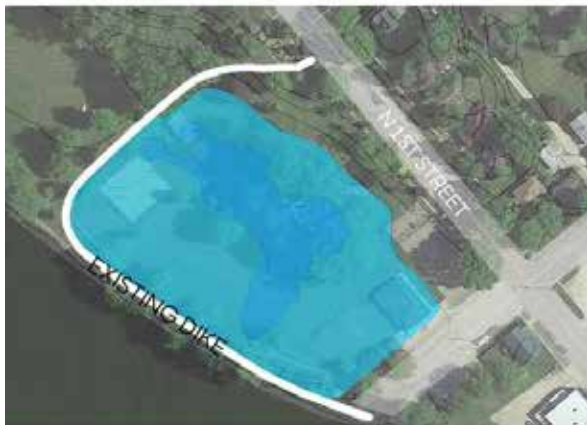
After flood waters recede, Perrin Park continues to be inundated with water due to the existing dike, which prevents the water from flowing back out
