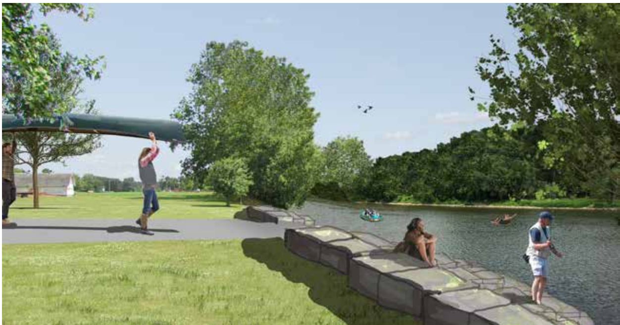
Image showing proposed changes in a FEMA buyout lot implementing brush clearing, stabilized bank treatment using limestone blocks, and a proposed canoe/kayak launch.
