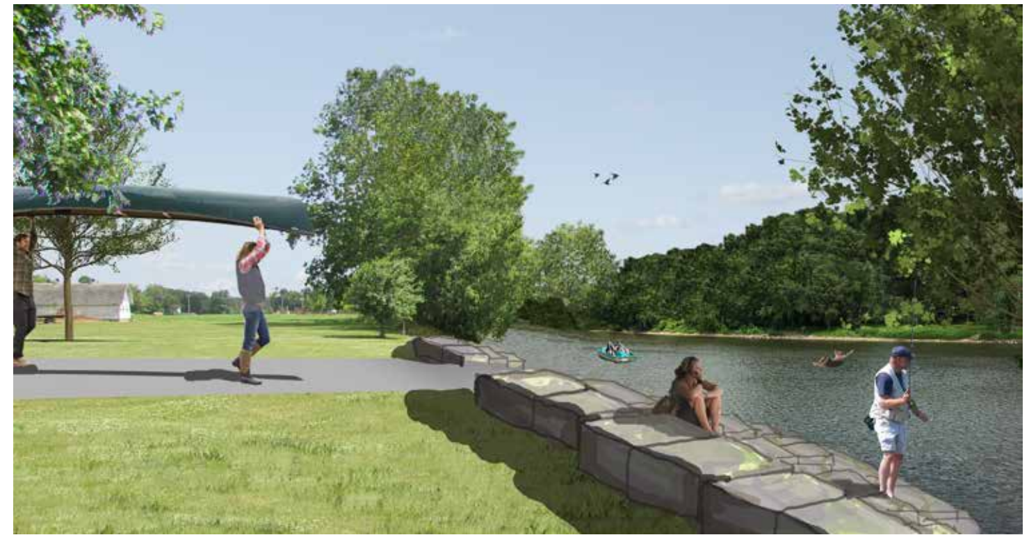
(After) Above image shows the conceptual design for treatment of the riverbank. Large stones armor the riverbank alongside a proposed canoe/kayak launch. A trail along the river connects to the canoe/kayak launch area.
