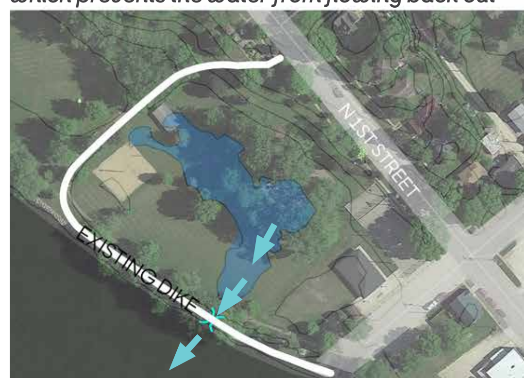
Installing a culvert with a back-up flap valve gate (pictured to the right) and grading the land to drain towards the culvert will enable the water to flow back out of Perrin Park and into the Shell Rock River
