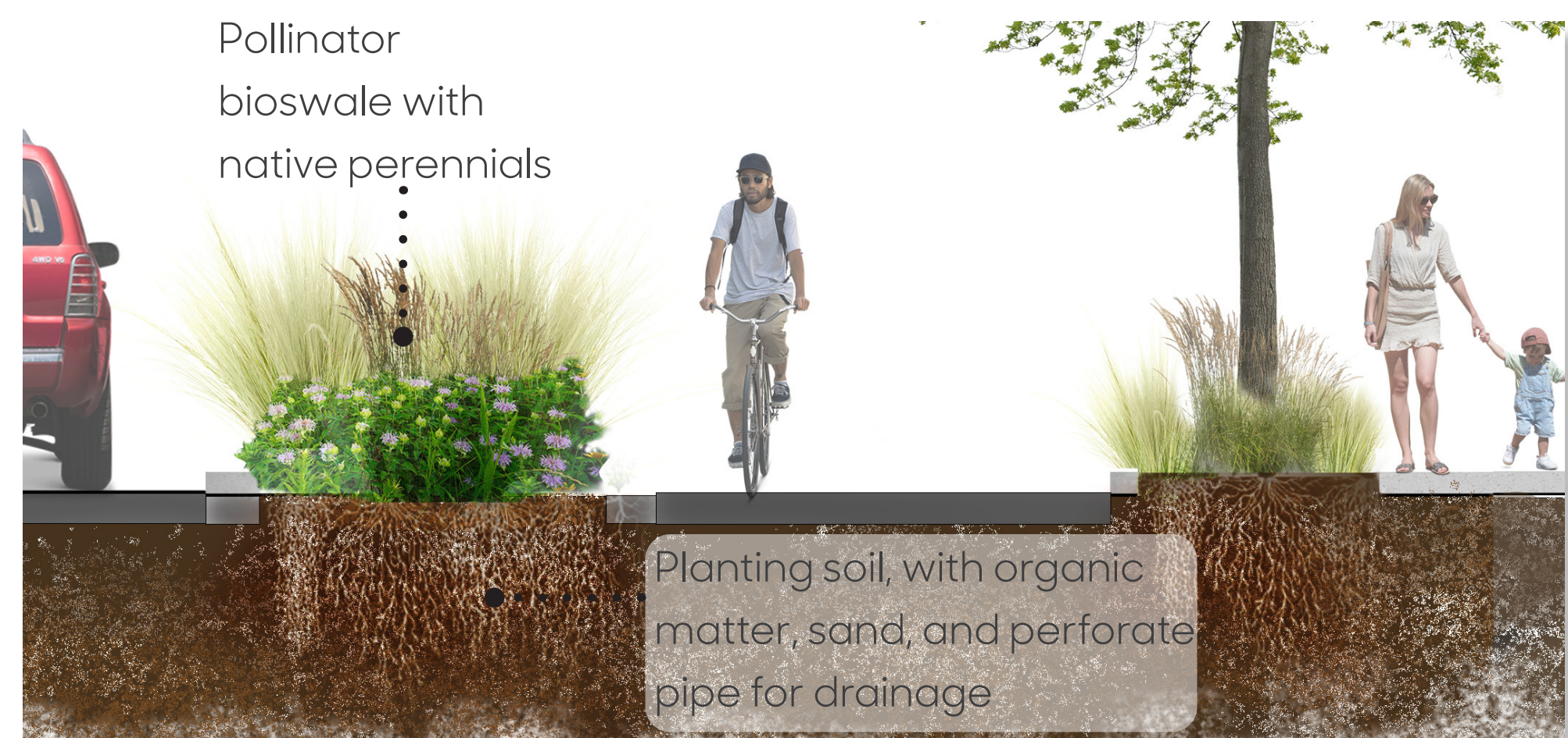
Bioswale Section
