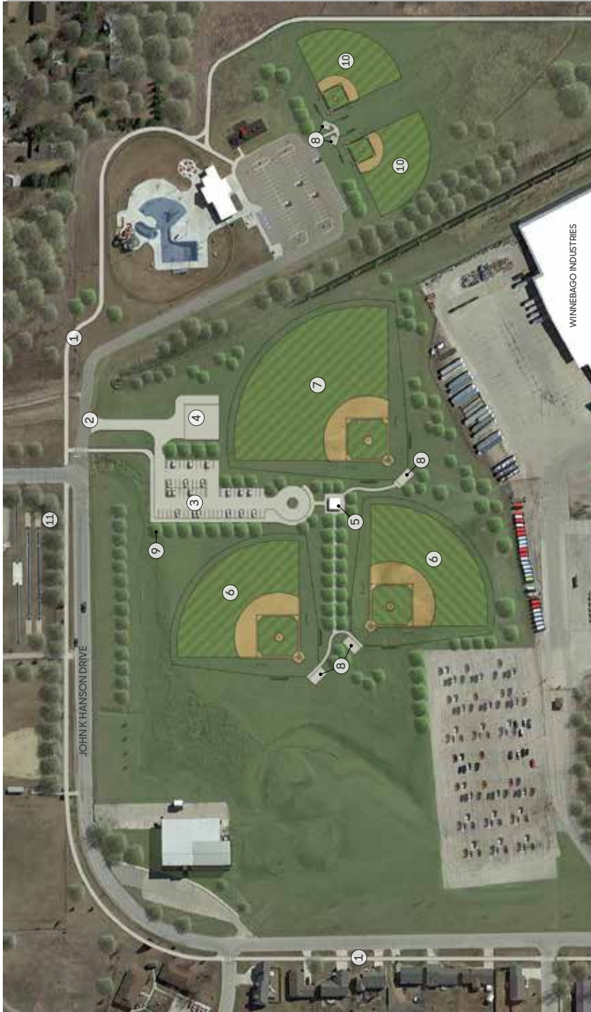
Site plan showing proposed baseball fields, circulation routes, trails, concession and restroom building, and shade tree plantings
