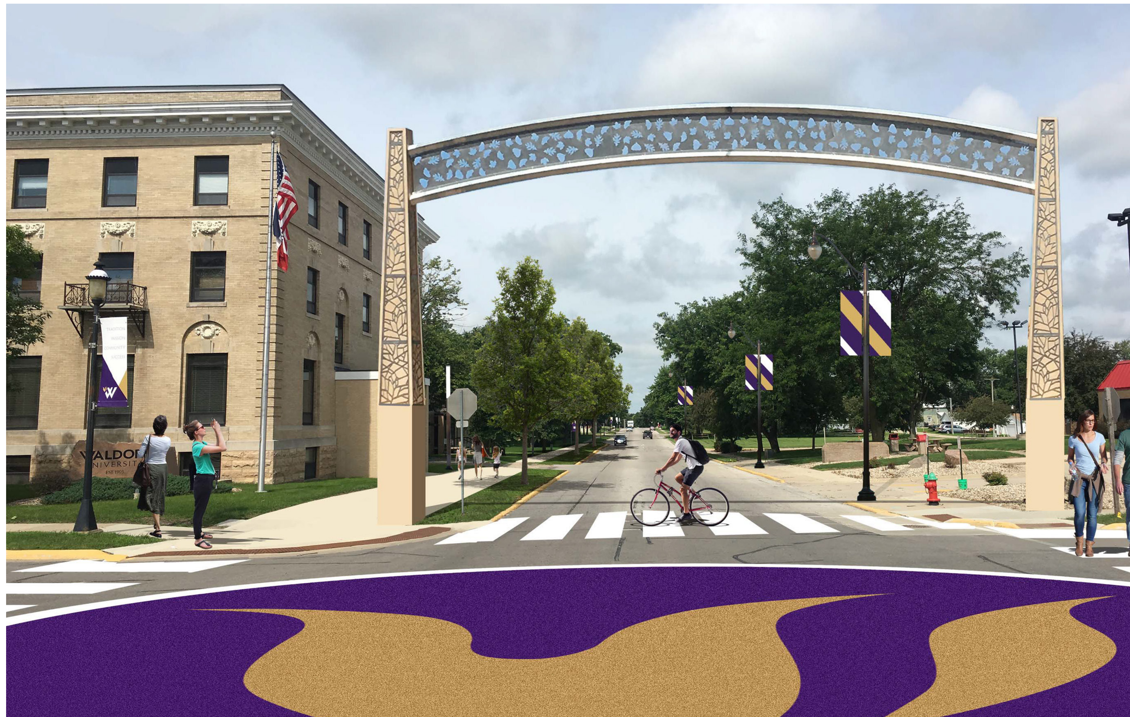
Proposed enhancements on J Street include reducing the width of J Street to include a 10' trail on the south side, tree plantings, art, improved lighting and highly visible crosswalks
