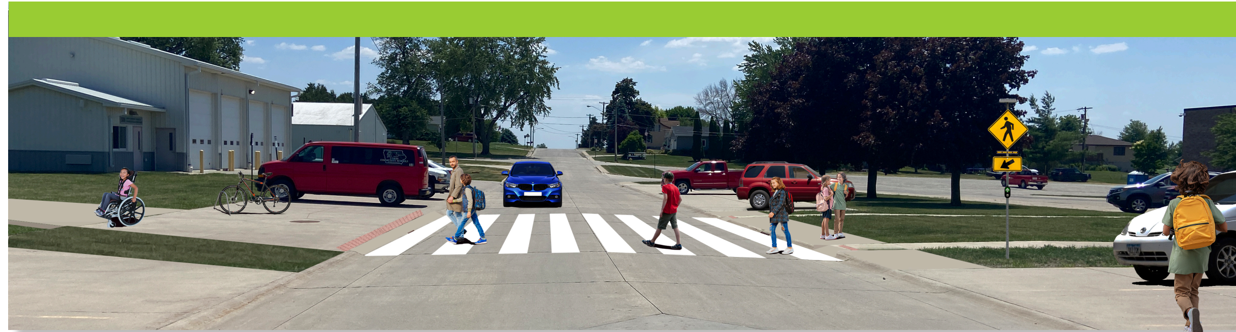
Proposed safety improvements at Union Middle School include a highly visible crosswalk, delineation of the trail and sidewalk from the parking area, tactile warning panels, and pedestrian crossing signage.
