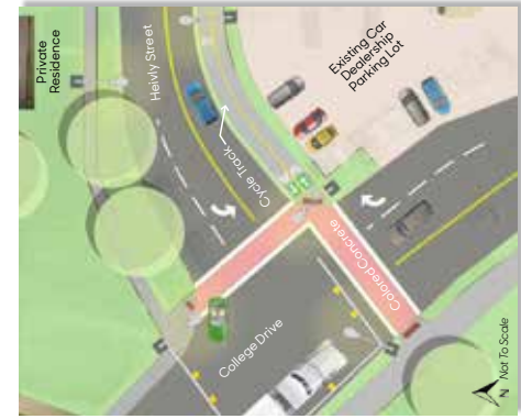
1 Plan view of College Drive and Healy Street showing optional intersection improvements with a protected two-way bike lane along the south side of Healy Street.
