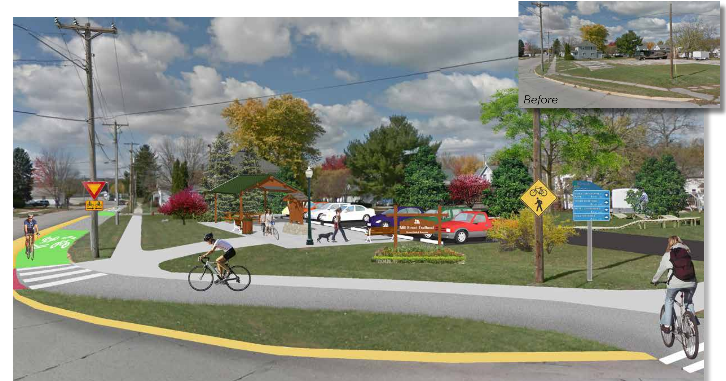
Perspective A showing the proposed two-way cycle track as it transitions to a separated trail at the Mill Street Trailhead.
