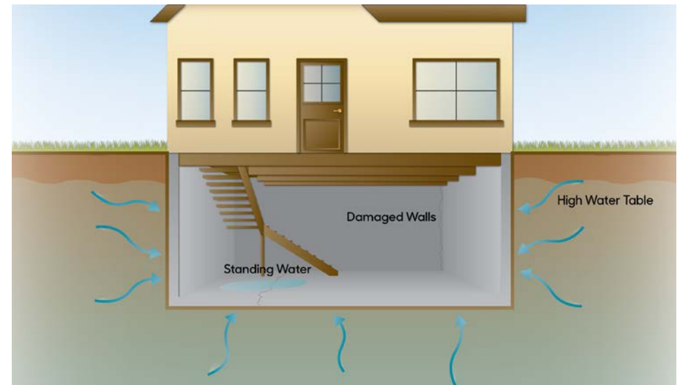
Diagram of the effects of a high water table on foundations and basements.
