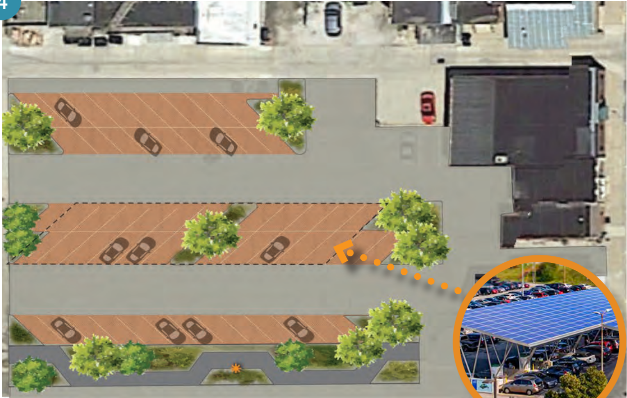
Parking lot layout highlighting zones for permeable pavers and vegetated biocells
